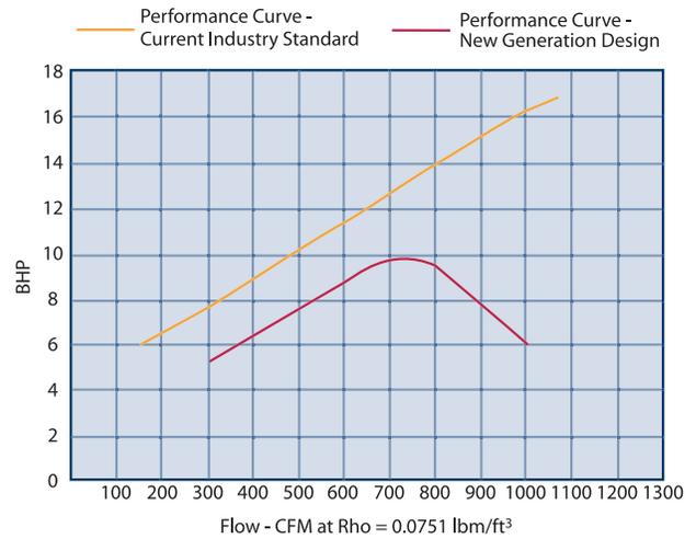
Figure 4 – Motor Power Comparison, units are matched in flow/pressure performance; new-generation product is matched to current industry standard performance curve via turn-down.
