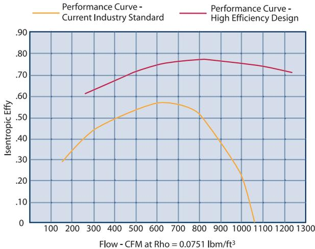
Figure 2 – Efficiency Comparison, units at constant 18,000 RPM impeller speed. Typical unit is at “0” Efficiency at 1,050 CFM because its discharge pressure is also 0 (see Equation 4 and Figure 1).
