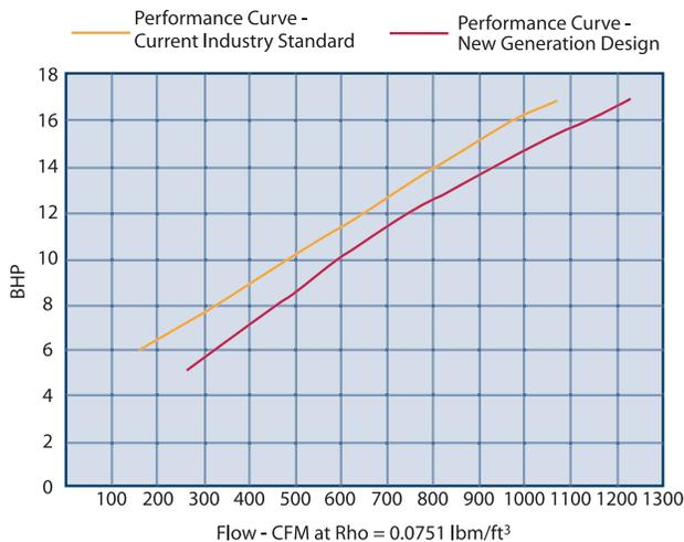
Figure 3 – Motor Power Comparison, units at constant 18,000 RPM impeller speed. Even though blower speed is the same, this comparison is misleading because pressure delivery, i.e., performance is not equivalent, as was shown in Figure 1.
