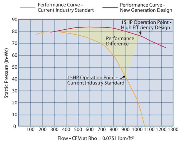
Figure 1: Direct Performance Comparison, units at constant 18,000 RPM impeller speed, with 15HP operating point defined for both. New-generation unit also delivers far greater performance for the same 15HP energy cost.
